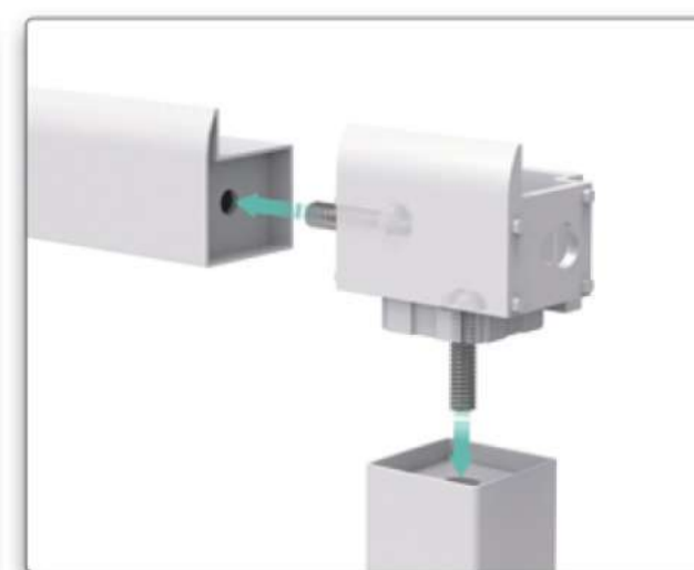
2 Assembly by screws
